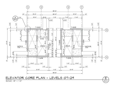
fig 4 – typical plan of shear wall core.
